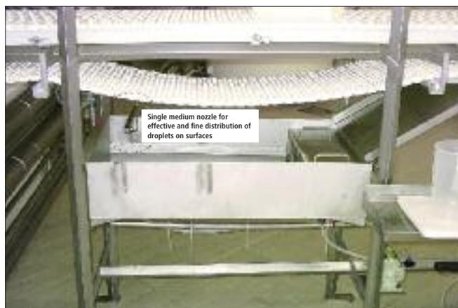
Single medium nozzle for effective and fine distribution of droplets on surfaces
