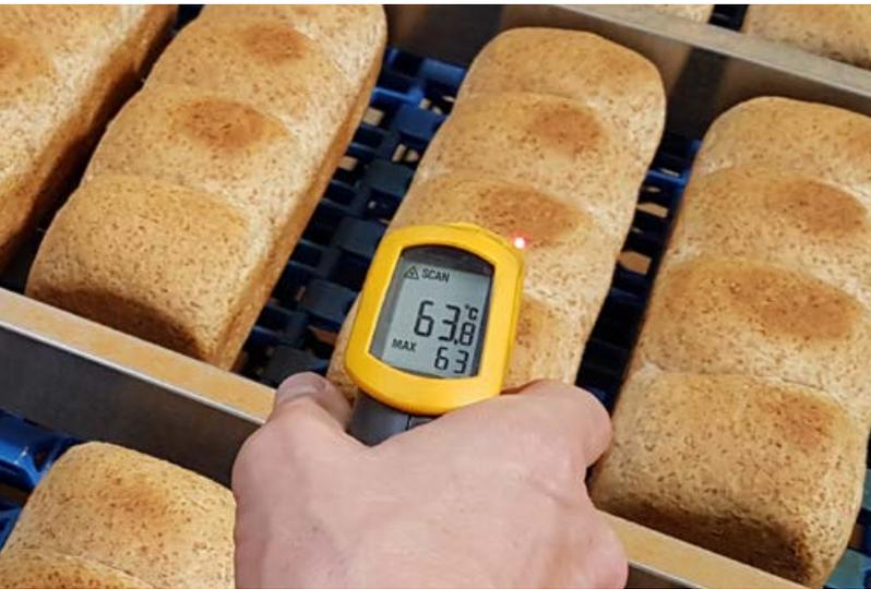
++ Monitoring the surface inflow temperature between baking-out and the cooling room
